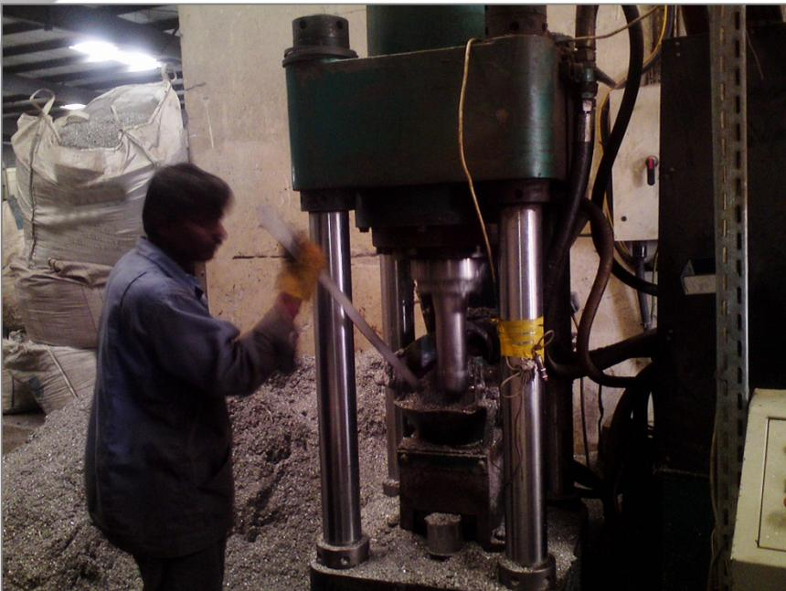
Manual "Material feeding" on the permanently open Chinese briquetting machine, photo taken by customer in April 2015
