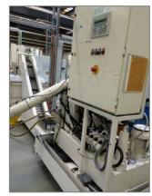
Another special feature lies in the construction concept: Both plants receive the shavings over spiral conveyers from a production centre, to which they are directly bound. In addition there is the possibility to fill the shavings externally via a hopper.
